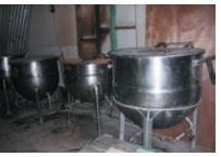
Locally made cooking and processing equipment were introduced so if anything broke down it could be easily repaired or replaced.
